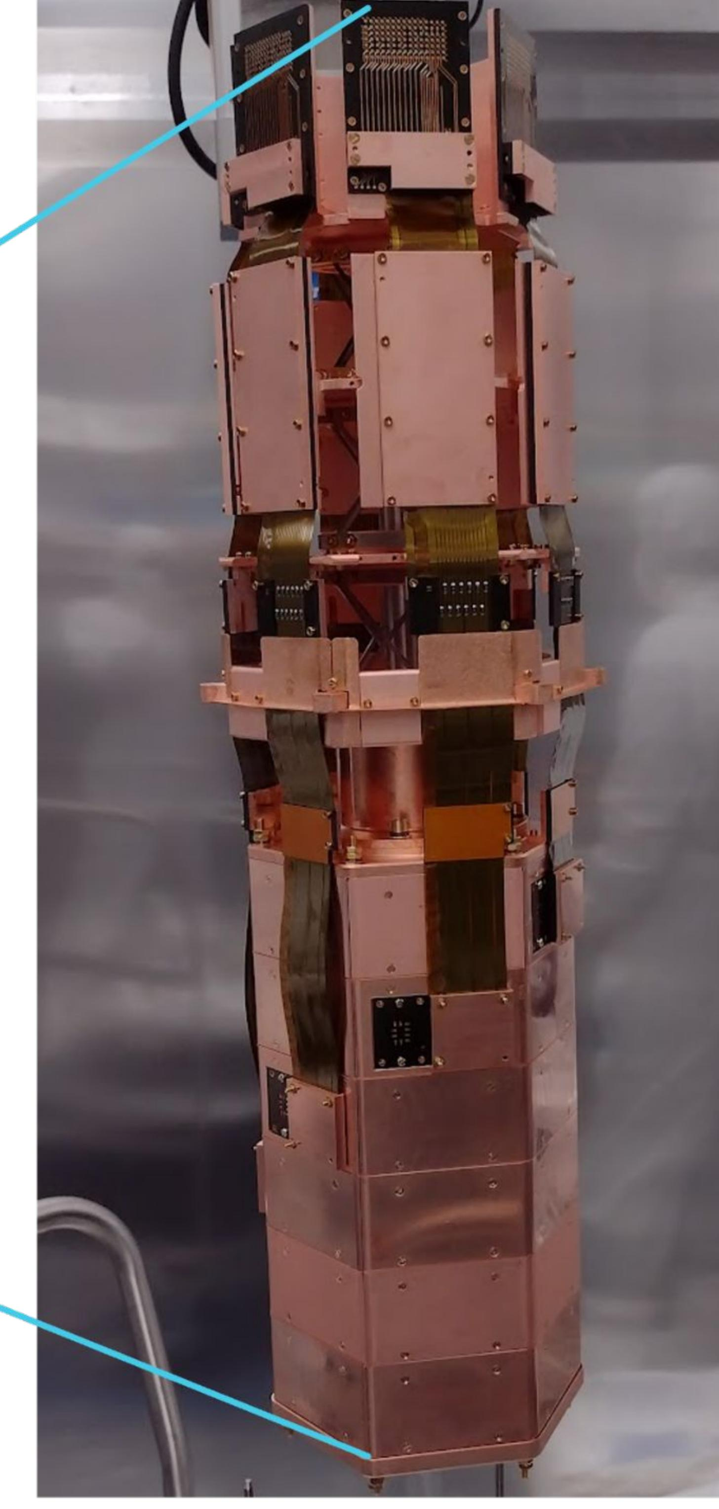
Detectors assembled in 4 towers, thermally coupled to each of the fridge stages
