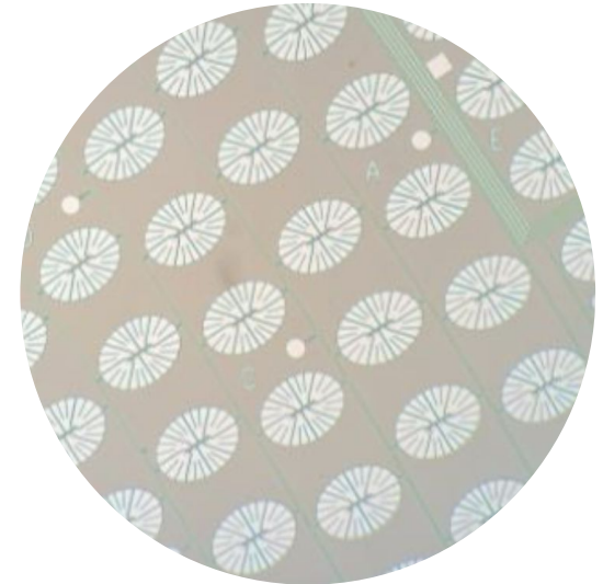
SuperCDMS TESs (500 \mu\text{m} long)
