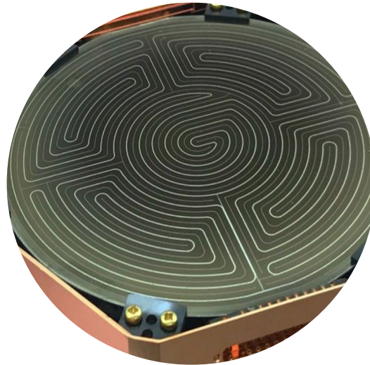
SuperCDMS charge sensor (10 cm)
